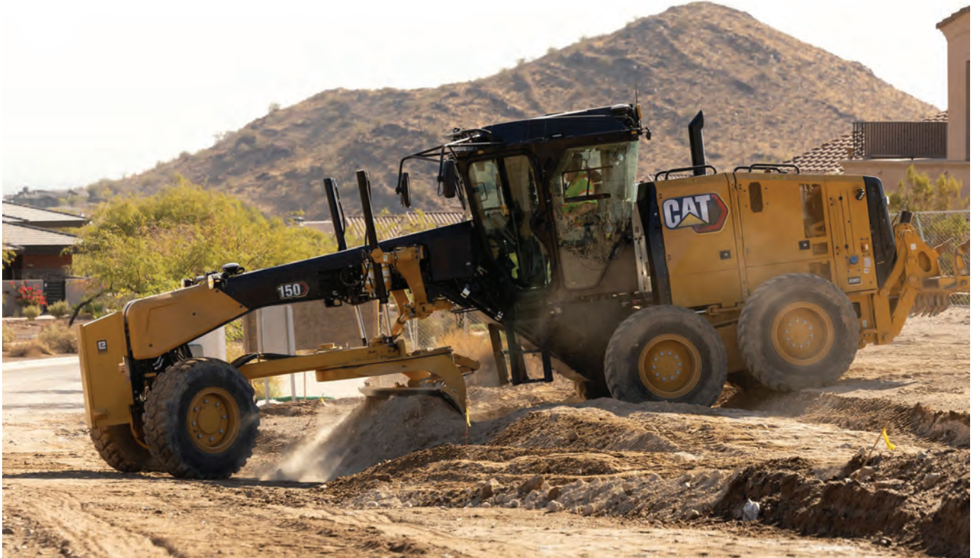
ABOVE AND BELOW: The fully redesigned cab features larger windows for enhanced all-round visibility, with particular focus on the mouldboard and tyres, while the 'operator-first' approach continues with improvements to HVAC and seat adjustment options.
