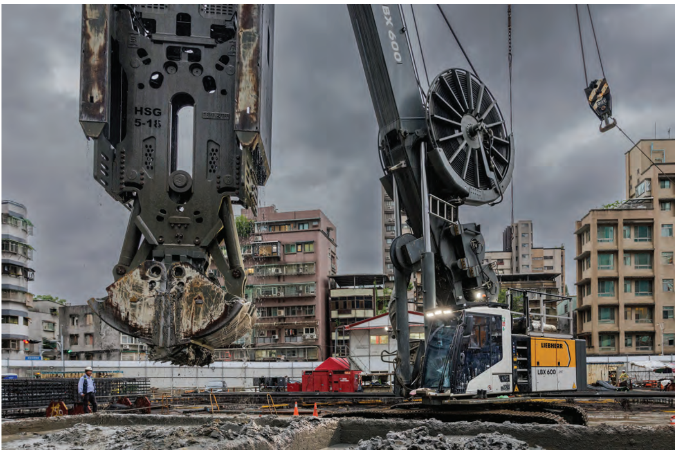
ABOVE AND BELOW: The standard version of the LBX 600 carrier machine features a total height of 17.8 m. For operations with limited headroom, work can be carried out in low-head configuration at 11 m or ultra-low-head configuration at 5.8 m.
