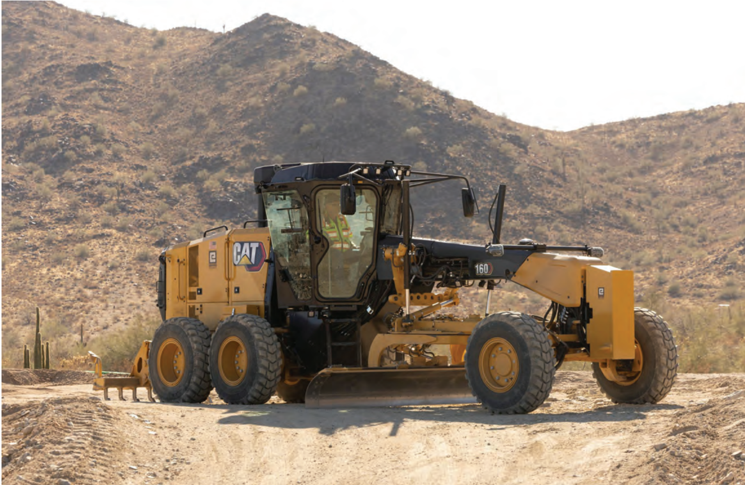
ABOVE AND BELOW: The fully redesigned cab features larger windows for enhanced all-round visibility, with particular focus on the mouldboard and tyres, while the 'operator-first' approach continues with improvements to HVAC and seat adjustment options.
