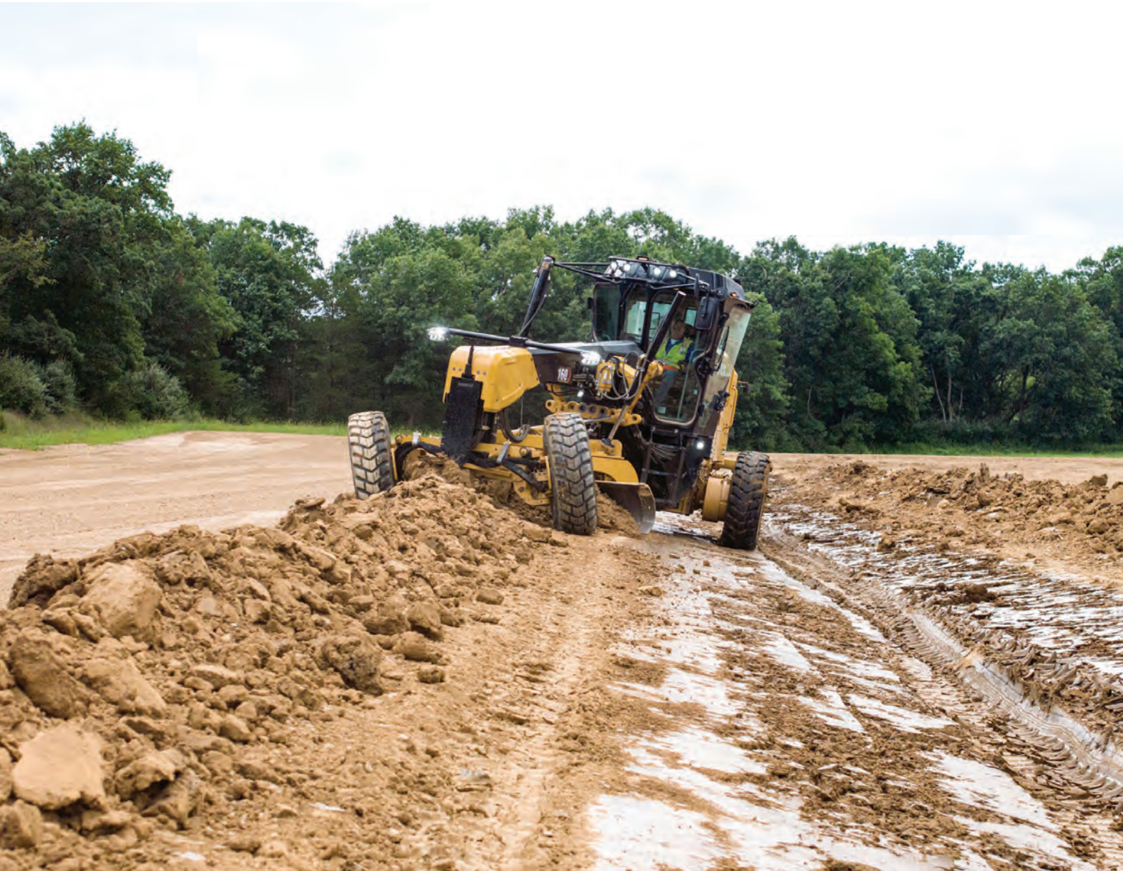
The Cat 150 and 160 motor graders come with 12-ft and 14-ft mouldboards, respectively. The easy-to-use joysticks place transmission, gear shifting and machine-direction control on the left, while the right handles drawbar, circle and mouldboard functions as well as throttle control and manual differential lock and unlock.
